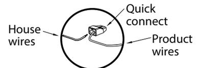
**NOTE:** Important wire information. Maximum temperature rating 221°F (105°C). 600 volts maximum for building wire and 1,000 volts maximum for building wire and 1,000 volts maximum in signs and lighting fixtures. The acceptable wire range includes: Solid: 12-18 AWG.
