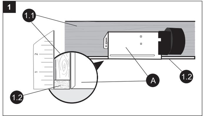
2. Mount the fan housing (A) to joist using the long wood screws (AA) on both sides.
