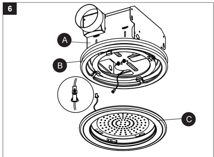
7. Place light/rim assembly (C) up to the light/rim assembly (B) and align the four rim locking buckles. Push light/rim assembly (C) into the light/rim assembly (B) and rotate counterclockwise until light/rim assembly (C) stops to lock into place.
