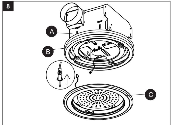
9. Place light/rim assembly (C) up to the light/rim assembly (B) and align the four rim locking buckles. Push light/rim assembly (C) into the light/rim assembly (B) and rotate counterclockwise until light/rim assembly (C) stops to lock into place.
